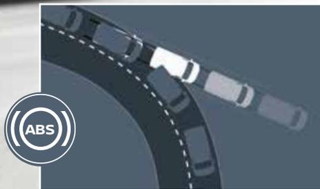
Anti-lock brakes help you retain steering control in emergency braking.
